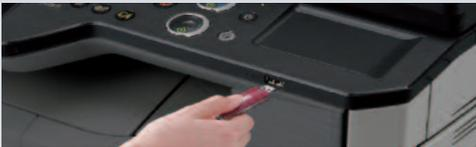
USB 2.0 port is located on the front panel for easy access\*
